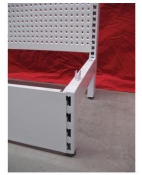
Put in the front kickboard. Adjust feet to make level and stable, repeat on other side as well, if double sided.
